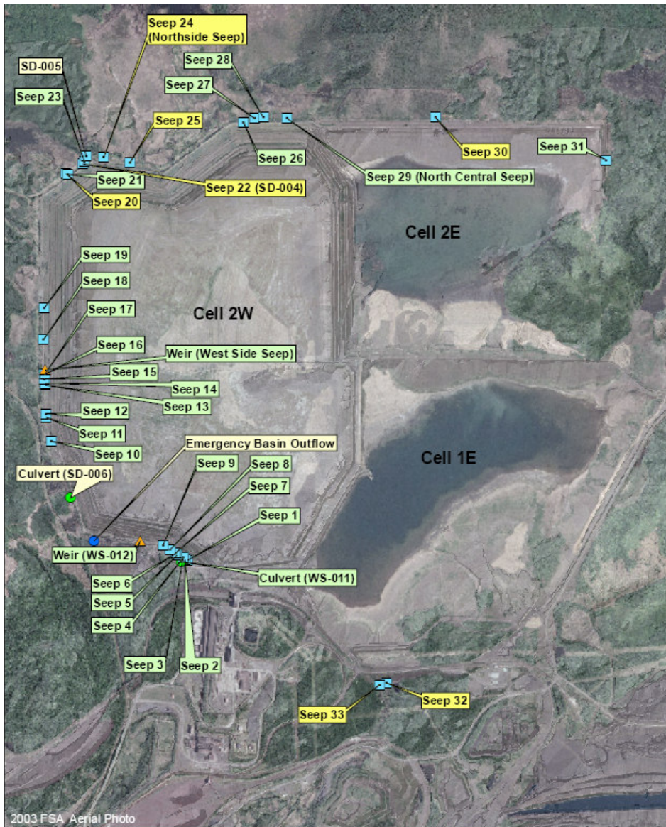
Figure 6 Seep Locations Tailings Basin
